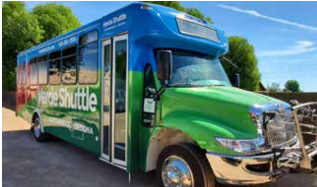
Pictured here is MPI 1105 full bus wrap with DOL 6460 PVC Free and SC950 Cut Vinyl lettering. Courtesy of VisionIt Media.
